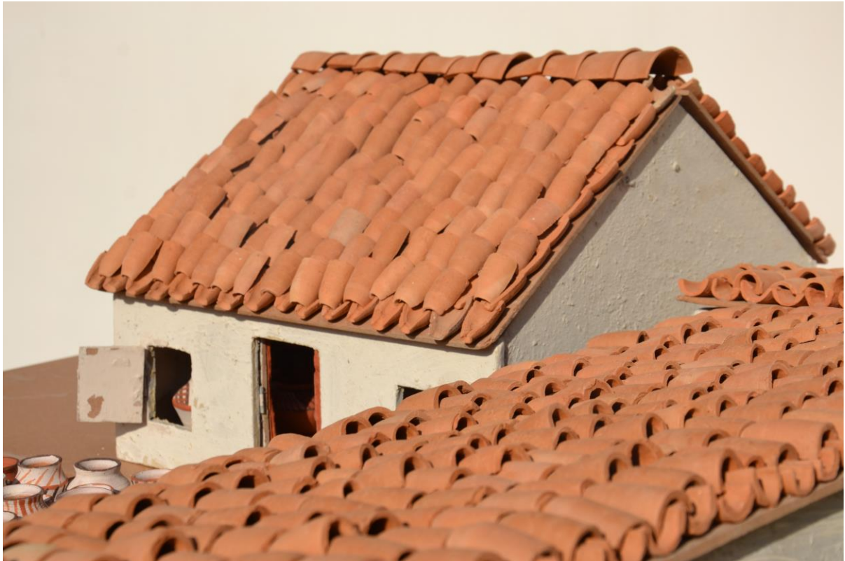
Figure.11 Prototype: Roofing System
